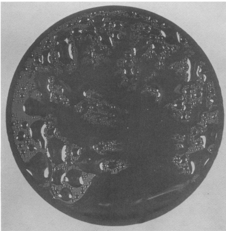
FIG. 4. Mixed filmwise and dropwise condensation results with a plating thickness equivalent to 300 layers of gold. This is Point C in Fig. 1.
